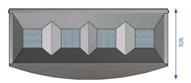
**Description:** Self-supporting, curved fronts, straight back and flat side panels made of stainless steel, secured with an internal construction of galvanized steel, provide great stability. The tops funnel-shaped openings guide waste into the inner liners and are also an elementary part of the fire protection (patented and certified).
