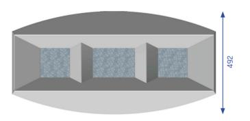
**Description:** Self-supporting, curved fronts and flat side panels made of stainless steel, secured with an internal construction of galvanized steel, provide great stability. The tops funnel-shaped openings guide waste into the inner liners and are also an elementary part of the fire protection (patented and certified).
