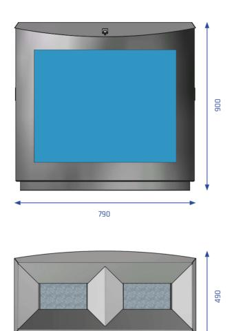
**Description:** Self-supporting, curved fronts and flat side panels made of stainless steel, secured with an internal construction of galvanized steel, provide great stability. The tops funnel-shaped openings guide waste into the inner liners and are also an elementary part of the fire protection (patented and certified).
