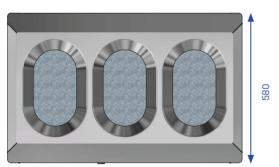
**Description:** Self-supporting, straight exterior walls incl. rounded corner profiles and a cover construction made of stainless steel, fastened with a galvanized interior construction, provide great stability. The funnel-shaped openings on the top of the container guide the waste into either a bag holder (version 1) or a galvanized inner liner, which also serves as a bag holder (version 2).
